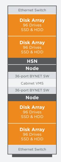
Figure 1. Teradata Active EDW 6750 Platform Cabinet Components.
