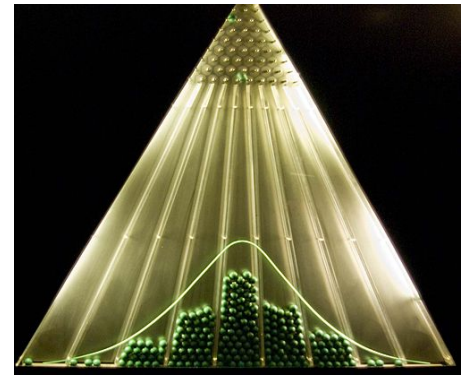
The bean machine , a device invented by Francis Galton , can be called the first generator of normal random variables. This machine consists of a vertical board with interleaved rows of pins. Small balls are dropped from the top and then bounce randomly left or right as they hit the pins. The balls are collected into bins at the bottom and settle down into a pattern resembling the Gaussian curve.
