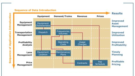
Figure 2. Potential data, application, and business benefits streams from an evolutionary data warehouse implementation and data mart consolidation for a rail network infrastructure business.
