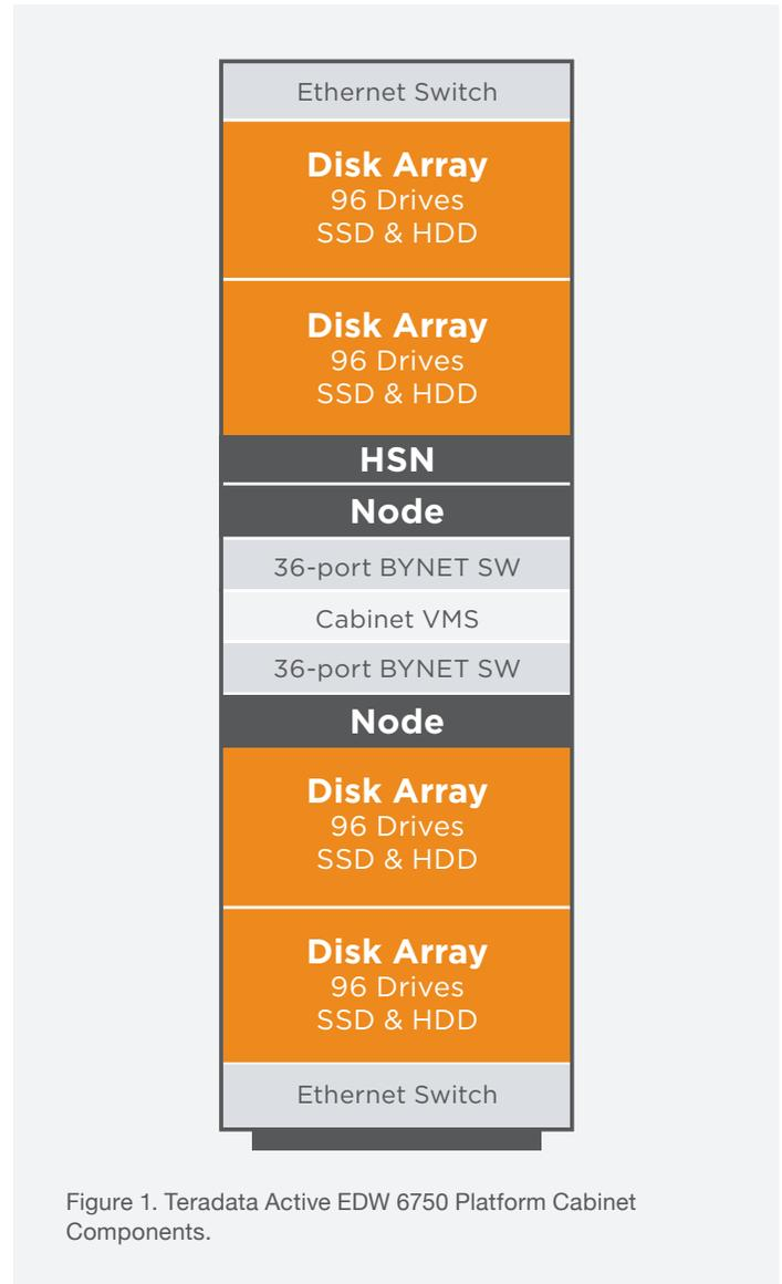
Figure 1. Teradata Active EDW 6750 Platform Cabinet Components.
