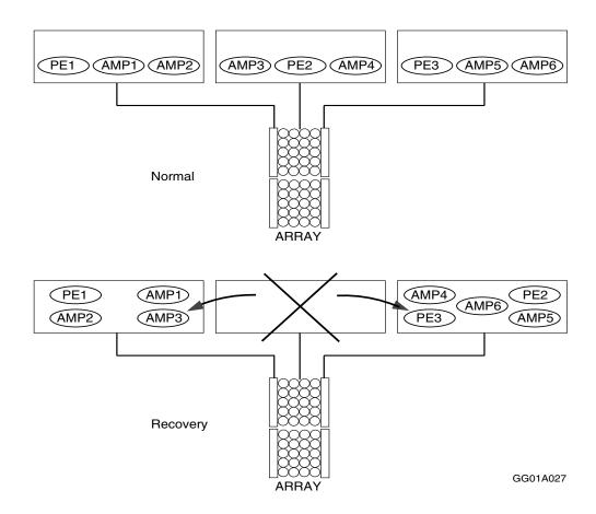
**Note:** PEs that manage TPA-hosted physical channel connections cannot migrate during a node failure because they are dependent on the hardware that is physically attached to their assigned node.
